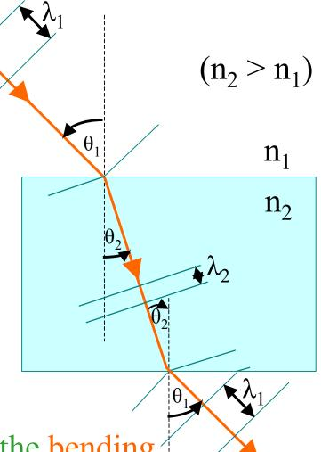
• Example of refraction: Viewing objects under water...
