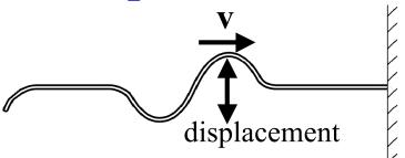
Pulse **propagates** down rope to wall **creating** an **instantaneous vertical displacement**.
