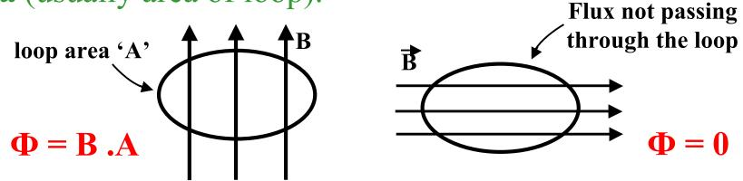
Maximum flux is obtained when field lines pass through circuit perpendicular to coil.
