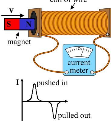
• Strength of deflection depended on number of turns on coil and on rate of motion of the magnet.
