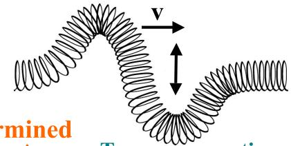
• Velocity of the 'pulse' is determined by the medium it is propagating in.
