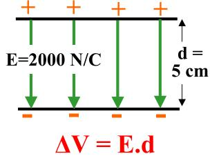
• The voltage will be maximum at the positive plate and will drop 100 V uniformly from top to bottom plate (i.e. it will be 50V in the center of capacitor).
