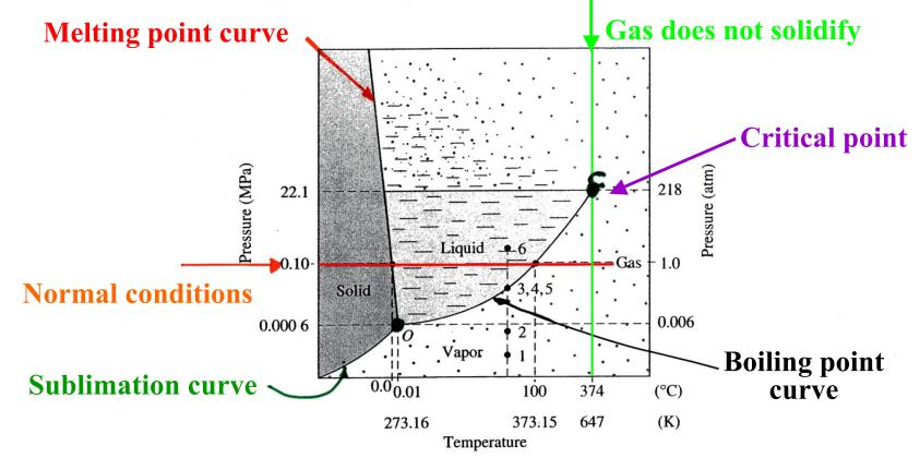
**"O" is triple point water** - solid, liquid and gas /vapor co-exist. Temp = 0.01 °C.
