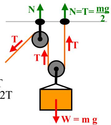
Key: The work done is the same for both the lifter and the object lifted as lifter needs to move 2d to lift object up 1d in height.
