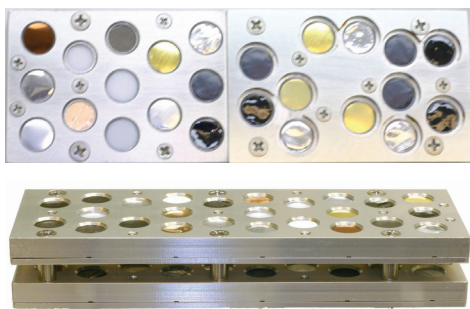
MISSE (Materials International Space Station Experiment) samples bound for 9-month deployment on the International Space Station.
