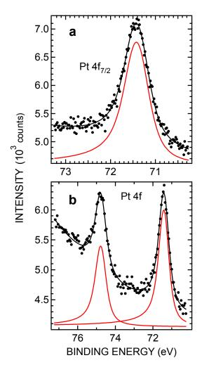
Fig. 3. Least-squares analysis of Pt 4f core-level spectra from the Pt/W(110) bimetallic interface for ~1 ML of Pt.
