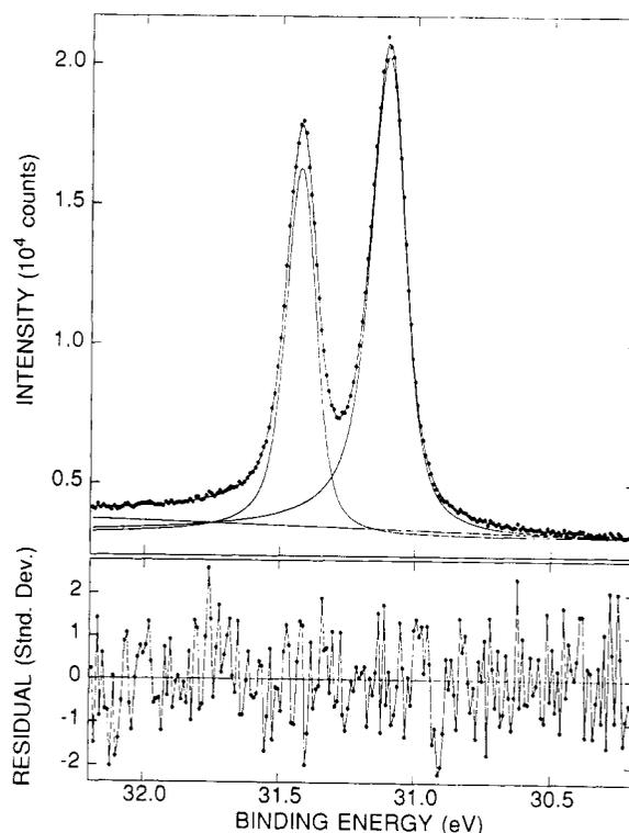
Fig. 3. Analysis of one of the W  $4f_{7/2}$  photoemission spectra of a clean W(110) surface. The data, taken with 70 eV photons, are fitted with a linear background and two fully independent lines, representing the surface (right) and bulk (left) contributions. The residuals of the fit are shown in the bottom panel.
