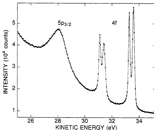
Fig. 2. Wide scan encompassing the  $5p_{3/2}$  and  $4f$  region of the W(110) surface, taken with 70 eV photons.
