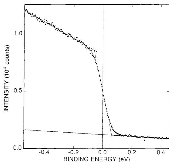
Fig. 1. The fermi edge of the W(110) surface at 210 K, taken with 70 eV photons and 40 meV electron analyzer resolution.
