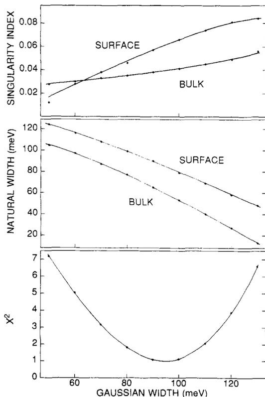
Fig. 4. Distinguishing between Gaussian and Lorentzian broadening. The bottom panel shows a cut through the Chi-squared surface of a least-squares analysis of the data in Fig. 3. The results were obtained by holding the Gaussian widths for both surface and bulk photopeaks to a common value and leaving the other parameters unconstrained. The corresponding natural Lorentzian widths and singularity indices are shown above.
