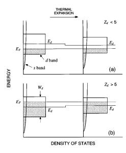
FIG. 4. Friedel model DOS illustration of the effect of lattice expansion on  $E_d - E_F$  for a *d*-band transition metal. Both  $Z_d < 5$  (a) and  $Z_d > 5$  (b) cases are illustrated. See text for details.
