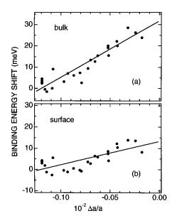
FIG. 3. Binding-energy shifts for the bulk (a) and surface (b)  $4f_{7/2}$  peaks of Ta(100) vs linear thermal expansion. The solid lines are linear least-squares fits through the experimental data points.
