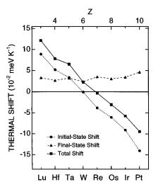
FIG. 5. Model calculation results for thermal core-electron BE shifts for the 5*d* transition-metal series. Initial state ( $\Delta E_{core}^i$ ), final state ( $\Delta E_{core}^f$ ), and the total shift ( $\Delta E_{core}^i$ ) are displayed for a 100-K increase in temperature.
