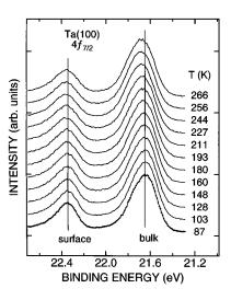
FIG. 1.  $4f_{7/2}$  core-level spectra of Ta(100) vs temperature. The vertical lines mark the low-temperature positions of each peak.
