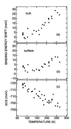
FIG. 2. Binding-energy shifts for the bulk (a) and surface (b)  $4f_{7/2}$  peaks of Ta(100) vs temperature. Also shown is the Ta(100) SCS (c) vs temperature.
