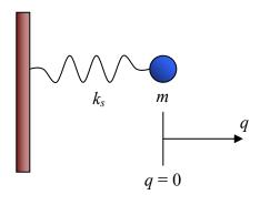
Note that the oscillator has only two parameters, the mass m and spring constant  $k_s$ . Assuming that the mass is constrained to move in the horizontal direction, its **displacement** q (away from equilibrium) as a function of time t can be written as
