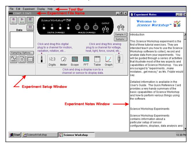
*Note:* **Before** you start Windows, connect the SCSI cable from the interface to the computer and turn on the interface power. You may connect the sensors at a later time. If not connected properly, *Science Workshop* will display the message "*Interface Not Found*".
