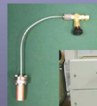
Fig. 7 Copper cylinder for graphite containment with tube for nitrogen gas, N 2 input.
