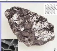
Fig. 5 a) Image of exfoliated graphite. b) Microscopic image of graphite. c) Illustration of graphite lattice structure—note the hexagonal planes. Images obtained from pubs.rsc.org , www.danajay.com , and www.benbest.com .
