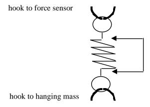
it.) Next, add a second 20 g mass and measure the new length (to the nearest mm). Remove the two 20 g masses and replace with a 50 g mass. Measure the new length. Add a 20 g mass; measure the new length. Finally, remove the 20 g and 50 g masses and replace with a 100 g mass. Measure and record the final length.
