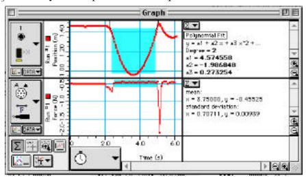
•E1.3 In the statistics panel for the force sensor data click and drag on the pull down menu and select Mean and Standard Deviation. Select the same time interval as for the position data. Record the mean value of the tension. Note the standard deviation value. That is a measure of how accurately the force sensor measures force. Most of the values in the interval shown will be within plus or minus one standard deviation from the mean value.
