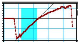
**acceleration.** (Why?) Select data over the first portion of "string only" motion as shown to the right. It should be clear that the velocity versus time does **not** have a single slope (as it should if the acceleration were constant throughout). Record  $a_2 (= a_u)$ . Select data over the second phase of the "string only" motion. Record  $a_2 (= a_d)$ .
