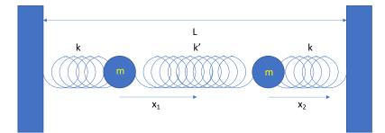
Each mass now feels two forces. We count forces to the left with a minus sign and to the right with a plus. On the left mass, positive  $x_1$  produces a force to the left,  $-kx_1$ , and when a force from the middle spring of  $k'(x_2 - x_1)$ . This second force is to the right when  $x_2 > x_1$  and to the left when  $x_2 < x_1$ . The equation of motion for the leftmost mass is therefore:
