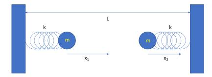
Suppose we have two identical mass-spring oscillators, each with mass m and spring constant k. (The masses and spring constants don't have to be the same, it just makes the example simpler) The oscillators satisfy
